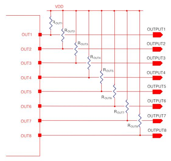
The OUTPUT pins have an open drain structure. For this reason, the connection of pull-up resistor R<sub>OUT</sub> is required between OUTPUT and VDD. The maximum output sink current is 4mA, so over a few  $k\Omega$  must be used as  $R_{OUT}$ . Normally  $10k\Omega$  is used as  $R_{OUT}$ .
