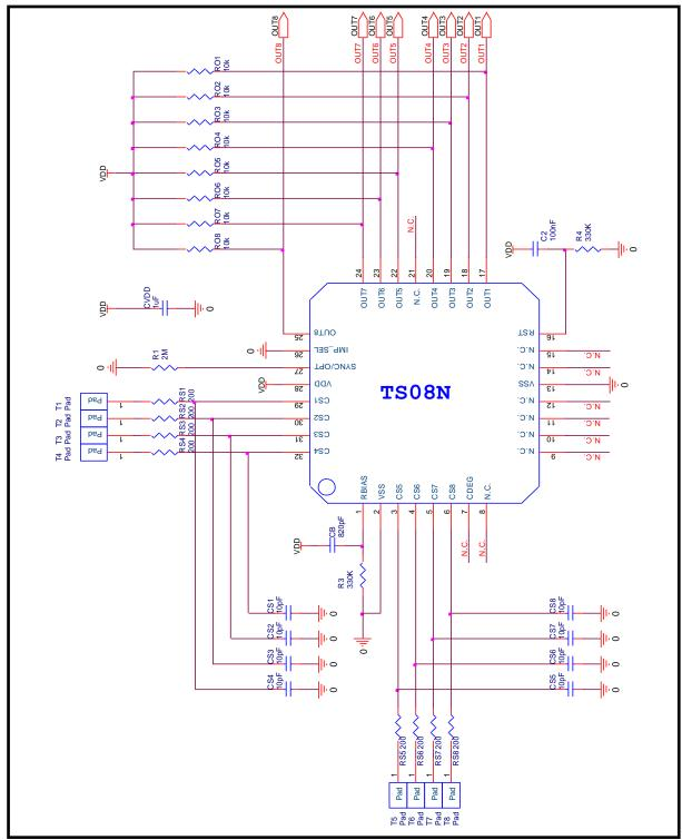
TS08N(32QFN) Application Example Circuit
