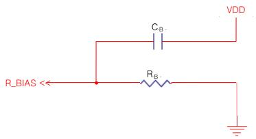
The R\_BIAS is connected to the resistor to decide the oscillator and internal bias current. The sensing frequency, internal clock frequency and current consumption are therefore able to be adjusted with R.B. A voltage ripple on R\_BIAS can make critical internal error, so C<sub>B</sub> is connected to the VDD (not GND) is recommended. (The typical value of C<sub>-B-</sub> is 820pF and the maximum Value is 1nF.)
