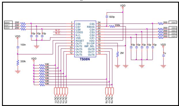
TS08N(24SOP) Application Example Circuit
